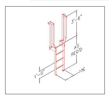
$ASP2436L-Attachable\ Ladder- \ \ \ ls\ designed\ for\ use\ with$  ASP equipment or work platforms or can be attached to parapet walls where accesses to heights are required. Shown here with optional handrail adaptors.
